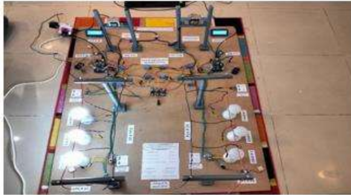
Figure 6.4 SLG Fault on Loads of PMT 1
